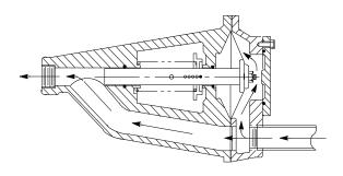
Figure 2. Valve in Open Position
